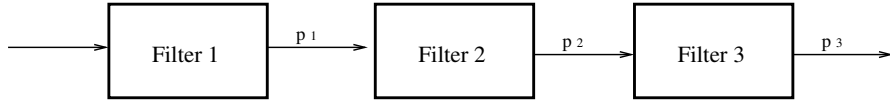
Figure 2: Searchlet Evaluation. The filters are applied, in sequence, to each object in the collection. The order of evaluation is chosen by the Diamond run-time environment. In the ordering above, Filter 1 is evaluated first, and passes p_1 of the objects to which it is applied. Filter 2 is evaluated next, passing p_2 of the objects passed by Filter 1; similarly, Filter 3 executes last, with a conditional pass rate of p_3 .
